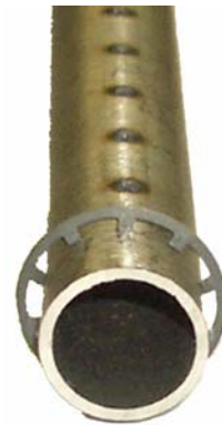
The "spring retainers" installed over the air tubes
